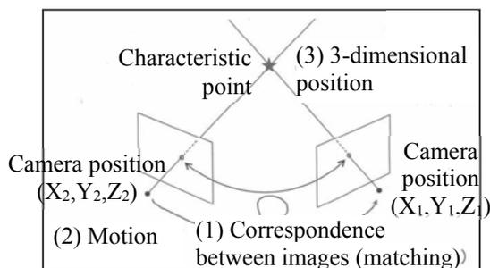
Fig. 2 Method of calculating characteristic point and camera position
