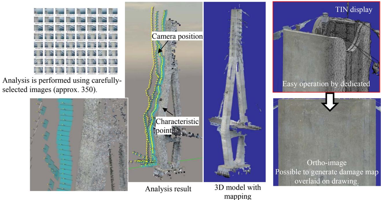
Fig. 15 Procedure from SfM analysis to generation of ortho-image
