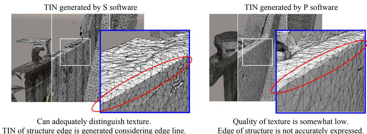
Fig. 5 Comparison of reproducibility of edge of concrete structure
