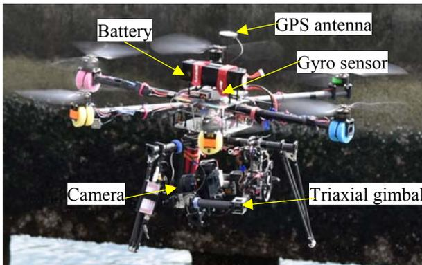
Fig. 6 Typical configuration of UAV (with camera attached)
