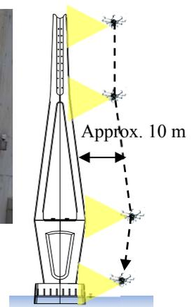
Fig. 11 UAV flight plan
