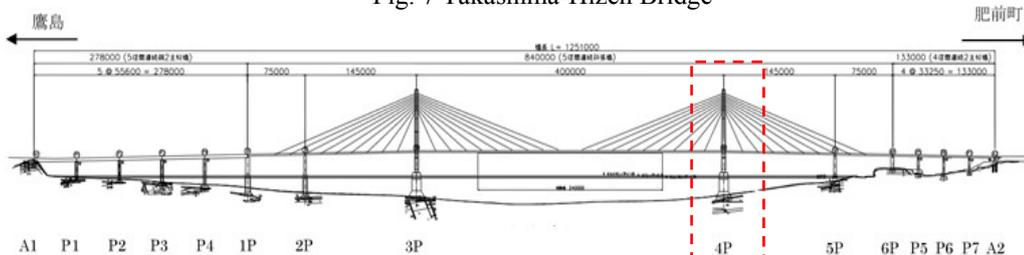
Fig. 8 Side elevation of Takashima-Hizen Bridge
