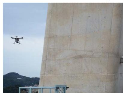
To photograph with a fixed focal point, photography is performed so as to keep a constant separation. → Instructions are given while monitoring transmitted images.
